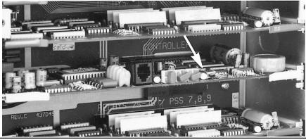
Individual Relay or Group of Relays Does Not Respond to the Test Switch (but does respond to direct switches) Turn off the low voltage power supply and reseat the Relay Driver Card(s) associated with those relays. Restore power and test. If still not working, turn off low voltage power and replace Relay Driver Card(s). Call the Emergency Number above for replacements.
