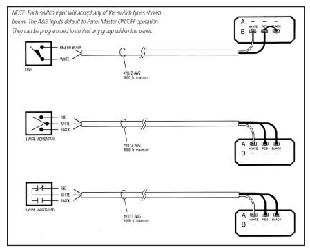
Wire Programmable System Switch Inputs
