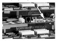
Press the Test Button on the RRC48 and hold for 4
